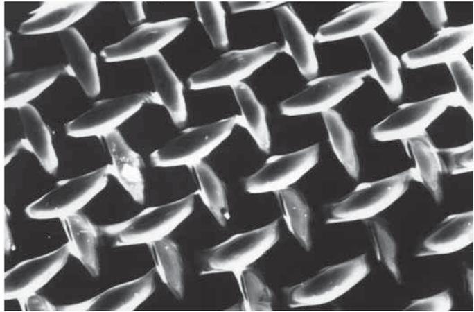
Nylon monofilament mesh
