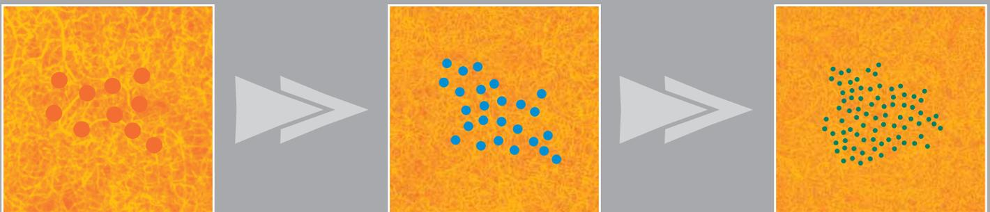
Within the extended life series, Allied Filter Systems Ltd is uniquely able to offer a **0.5 micron polyester** filter bag. The filter media has a special construction using a blend of micro denier and fine denier fibres, giving the finest filtration results of any needlefelt product available on the market.
