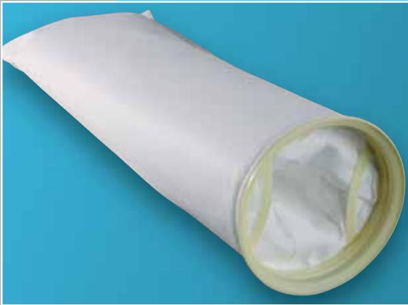
The multi layered construction provides an exceptional depth of filter media, around 50mm. The layers of oil absorbent media are separated by drainage layers, ensuring a good flow of liquid and minimising the pressure drop across the filter bag. The outer layers of the filter provide an effective final filtration of the process fluid, retaining very high levels of solids. Particle retention is >95% at the stated micron rating.
